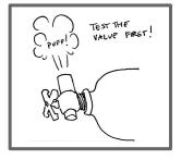
Test the valve, and lay the tank on the ground. Attach the regulator if one came with your tank (not pictured).
