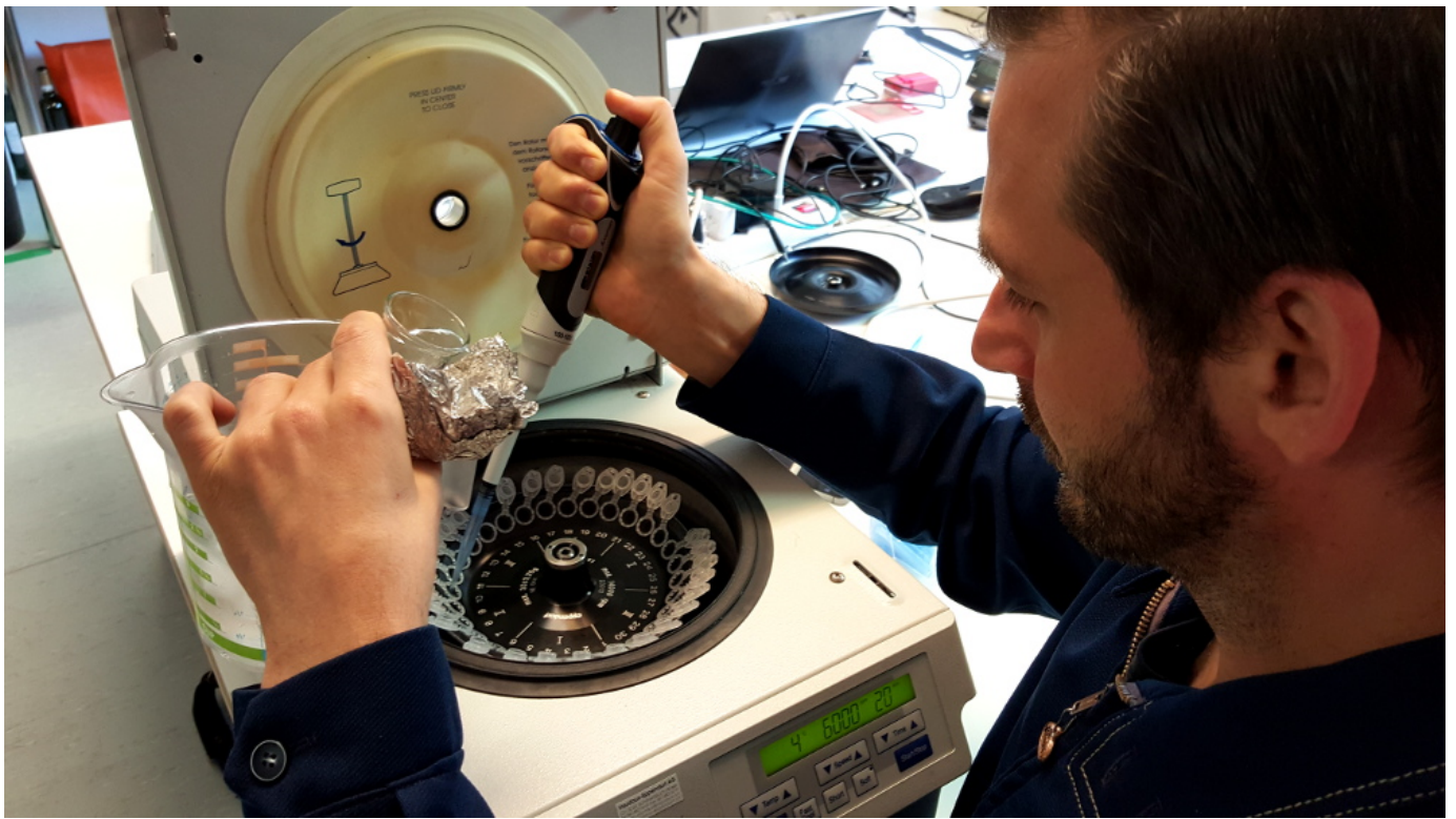
Centrifuge bacteria in 40 eppendorf tubes, remove the supernatant, add TSS buffer resuspend the cells
