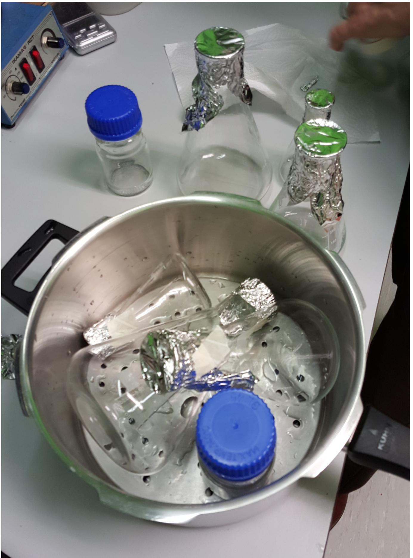
Sterilization of glass ware. Cover the top of flasks with aluminium.
