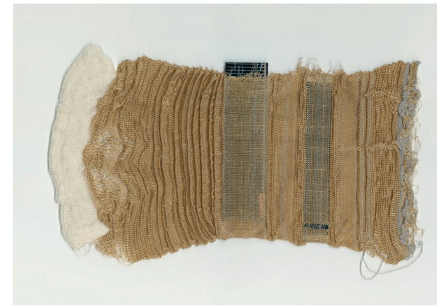
knitted trial with integrated photovoltaics
