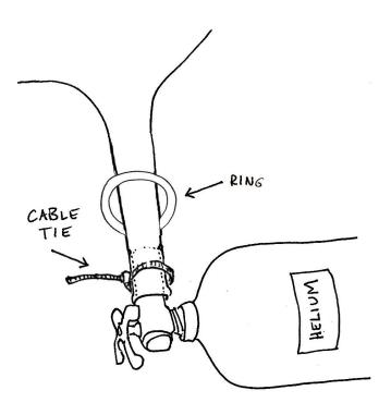
3. When you're done filling, push helium up out of the neck and close it with a removable zip tie (cable tie) or a very tight but untieable knot (shoelaces work well) just below the balloon.
