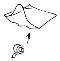
Where available, emergency mylar sleeping bags can be taped shut and, if carefully sealed, can stay filled for several days, unlike weather balloons. Two of these are enough to lift a typical camera.
